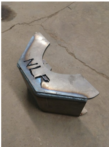
Example for type of cradle allowed and pulley protector.
