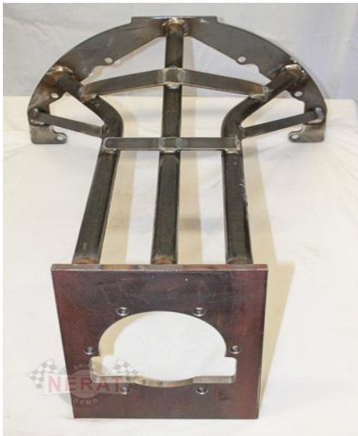
Example of trans braces allowed.
